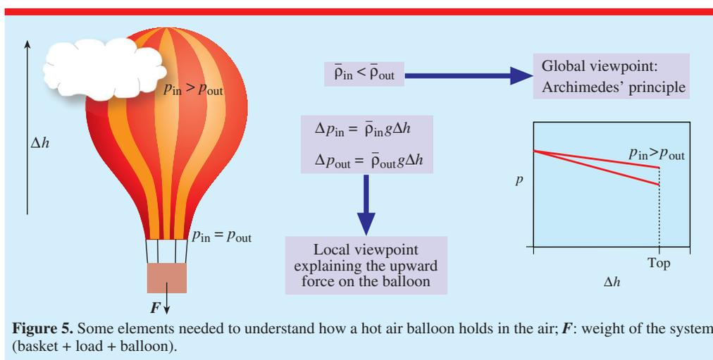
**Figure 5.** Some elements needed to understand how a hot air balloon holds in the air;  $F$ : weight of the system (basket + load + balloon).
