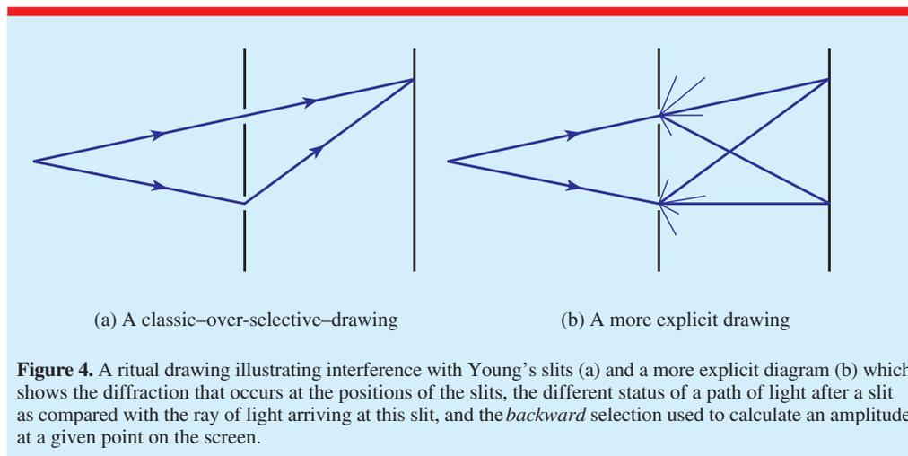
**Figure 4.** A ritual drawing illustrating interference with Young's slits (a) and a more explicit diagram (b) which shows the diffraction that occurs at the positions of the slits, the different status of a path of light after a slit as compared with the ray of light arriving at this slit, and the *backward* selection used to calculate an amplitude at a given point on the screen.
