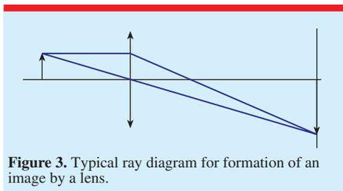
**Figure 3.** Typical ray diagram for formation of an image by a lens.
